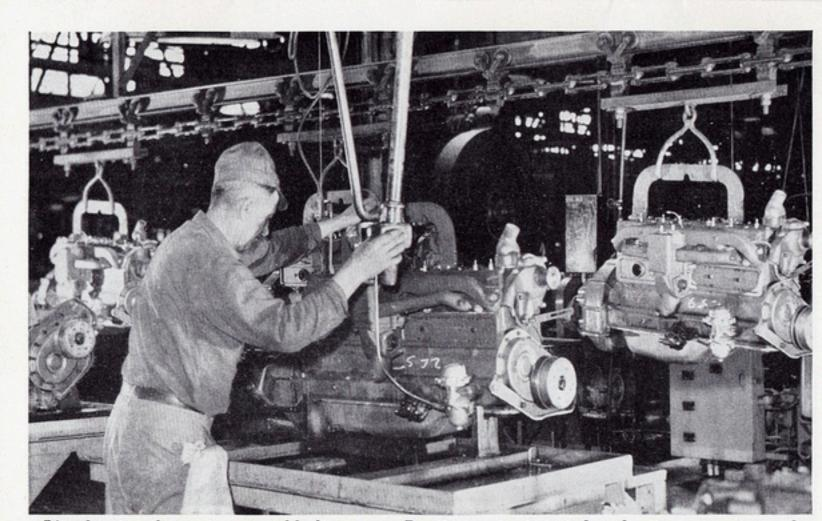
After leaving the motor assembly line, every Pontiac motor is tested under its own power and adjusted for perfect operation
